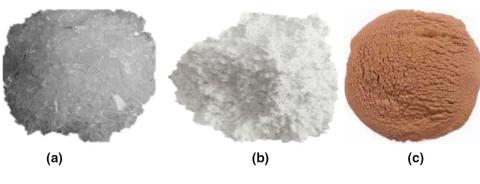
Fig. 2 Prepared composite sheets a pure polyester sheet b ZnO/polyester nanocomposite c Pure polyester/ZnO/CSNF Composite
