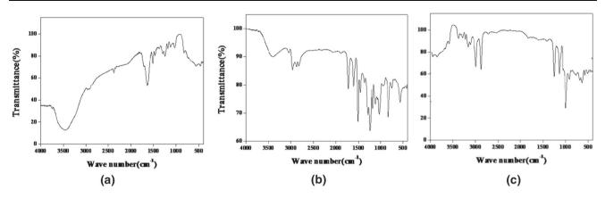
Fig. 4 a FTIR spectrum of pure Polyester b FTIR spectrum of Polyester + 1% wt ZnO b FTIR spectrum of Polyester + 1% wt ZnO + 1% wt CSNF
