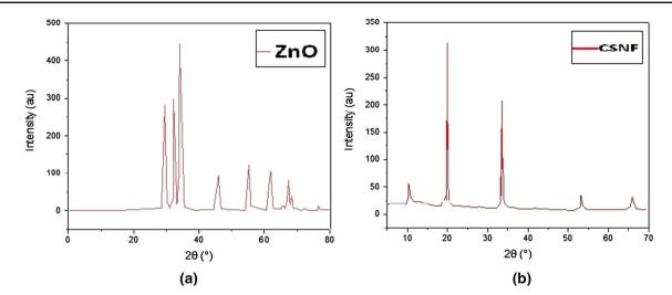
Fig. 3 XRD Results of a ZnO b CSNF
